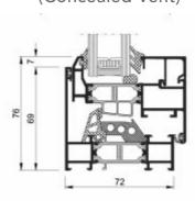
Narrow sightlines with visible aluminium facet on the vent
