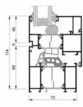
Straight overall contour with flush vent and frame line
